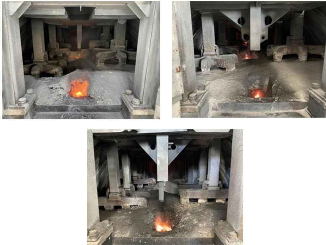
Figure 1. The condition and the thickness of the covering material on the anode of each potline.
